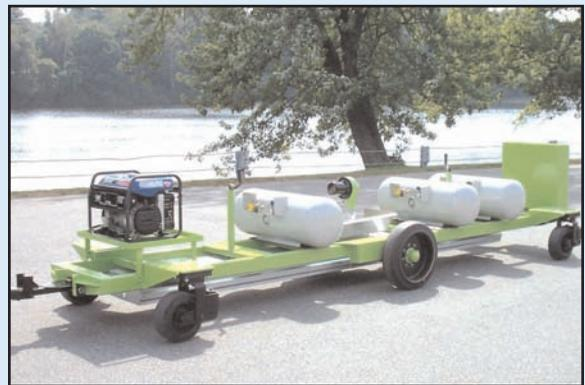
The patented **Ray-Tech Joint Heating System** effectively eliminates longitudinal cold joint failure by providing 98-100 percent density at the joint. The infrared heating system is capable of in-depth heating of longitudinal joints without burning or damaging the asphalt. This complete system is a proven, effective method of eliminating joint failure.
