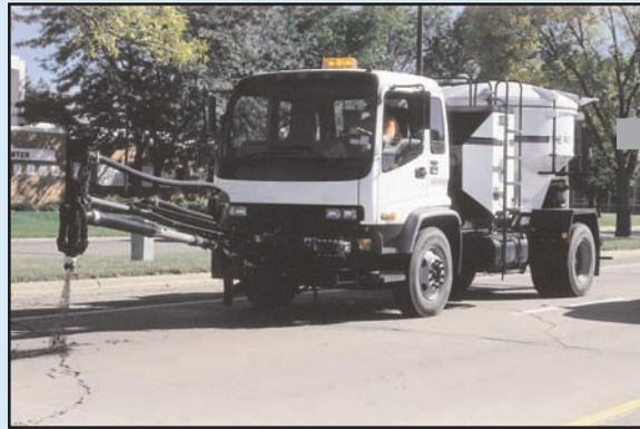
The **Rosco RA-300 Spray Injection Patcher**, with its one-person, from-the-cab operation makes safely and effectively repairing potholes a year-round activity. The RA-300 features its in-cab controls, full-function spray nozzle with joystick control and front-mounted patching boom and rear-mounted arrowboard for maximum simplicity, effectiveness and safety. Its hydraulic "Patch-on-the-Go" feature allows for patching on the move with no auxiliary power.
