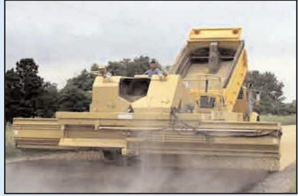
**Etnyre Chip Spreaders** are designed to spread aggregate in the chip seal process. The spreaders feature controlled application rates and have individual one foot wide power gates across the entire spreader width. Engine options range from 200 to 240 hp and the chip spreaders are available in front wheel or four wheel drive models.
