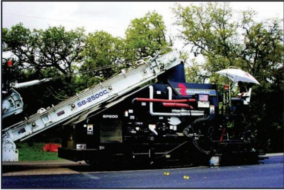
Roadtec's **SP-200 Asphalt Spray Paver** allows asphalt cement or emulsion (tack) to be sprayed directly in front of the asphalt mix before it is laid. Spraying the tack only seconds before the asphalt is laid provides a strong bond between the existing surface and the new pavement, which is especially important with thin overlays. The SP-200 also eliminates the need for separate tack trucks and does away with the inconvenience of tack adhering to tires of other construction vehicles.
