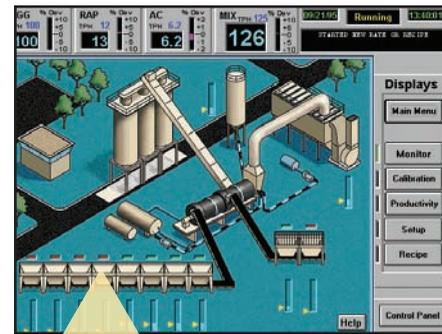
*Graphical user interface (GUI) for control of an asphalt plant*
