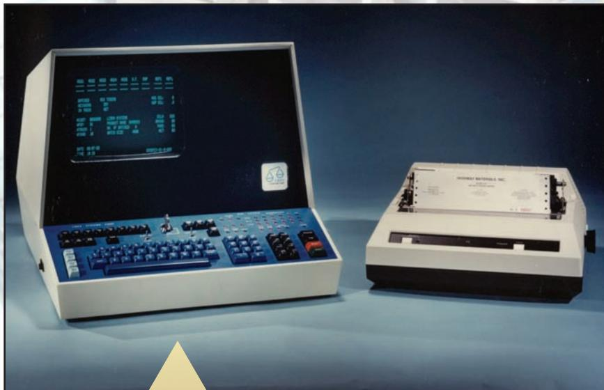
*EPROM-Based Asphalt Batching System, circa 1977*
